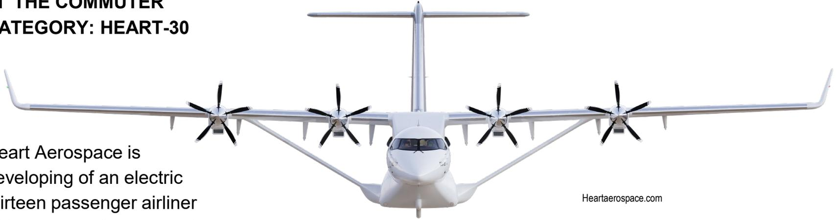
Heart Aerospace is developing of an electric thirteen passenger airliner with an operating range of 400 km, so commuter type of aircraft, with the goal to deliver the first unit fully certified for commercial flight by 2028. Aernnova is part of this project.
